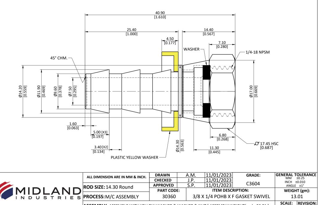
ASSEMBLY: ASSEMBLE WITH YELLOW WASHER & WASHER & NUT [ ASSEMBLY WEIGHT(gm) : 26.01 ] SCALE: N.T.S.
