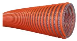
APPLICATION:GOOD FOR BOTH SUCTION AND DISCHARGE APPLICATIONS, THIS HEAVY DUTY HOSE CAN BE USED FOR RENTAL/CONSTRUCTION PUMPING AS WELL AS FISH SUCTION HOSE. COVER:Clear abrasion and weather resistant PVC. REINFORCEMENT:Orange PVC helix with high tensile synthetic textile yarn. TUBE:Smooth clear PVC. TEMPERATURE:-23C to +65C(-10F to +150F)
