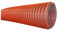
APPLICATION:GOOD FOR BOTH SUCTION AND DISCHARGE APPLICATIONS, THIS HEAVY DUTY HOSE CAN BE USED FOR RENTAL/CONSTRUCTION PUMPING AS WELL AS FISH SUCTION HOSE. COVER:Clear abrasion and weather resistant PVC. REINFORCEMENT:Orange PVC helix with high tensile synthetic textile yarn. TUBE:Smooth clear PVC. TEMPERATURE:-23C to +65C(-10F to +150F)
